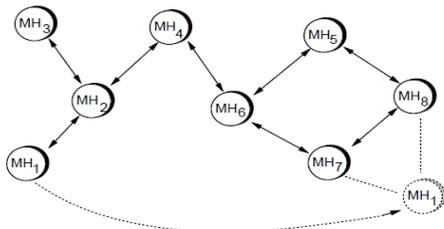
Figure 4.1: Movement of Mobile host in Adhoc Networks
